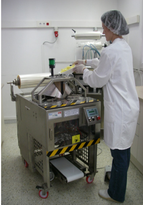
SOST-CO2 – Vertical form fill seal machine (VFFS) for modified atmosphere packaging of food.
